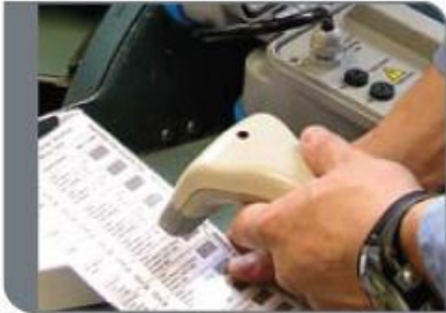
Bar code support for test data and tested appliance name entering.
